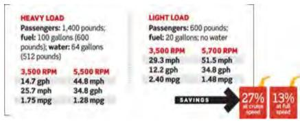
Next, we ran the Bluewater "light." We drained the fuel down to 20 gallons. We stripped it of every bit of gear but for required safety equipment — and, yes, discovered we had more on board than we'd need on any three fishing trips. Then we set out with a three-man crew weighing 600 pounds and increased our economy by a whopping 27 percent.
