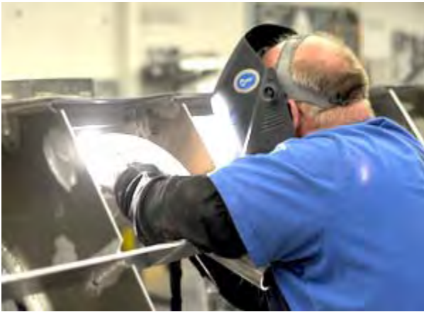
A welder pieces together an aluminum RB-M keel. Photo by PA2 Dan Bender
